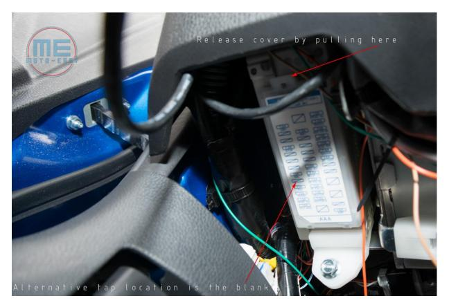
Alternatively, you can do a permanent installation by tapping the blue/red wire.
