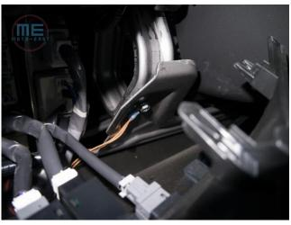
Locate the fuse box. Insert the supplied tap into the 7.5 AMP Gauge slot, or any powered slot (powered only with ignition ON). Re-use the 7.5 amp fuse, and take a 7.5 amp fuse from the spares in the underhood fuse box (or get a new 5a fuse). Combine this wire with the ORANGE wire from the sensor harness. Insert into crimp on the ECA harness and crimp down. Melt the heat shrink to secure wiring.
